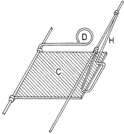
Figure 2.—Closed door of trap locked into place by a wire hook.
